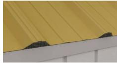
Step 3: Place the roof panel over pre-cut closure configuration for a snug fit. Attach panel over closure with Marco QuikGrip™ or QuikDrill<sup>™</sup> fasteners.
